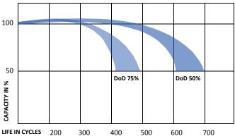
\* Cycle life is measured with a discharge current 0,2C, charged 16h and rest capacity of 2/3 Cn
